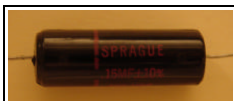
A later model Black Beauty, distinguished by red markings and lack of a filler tube.
