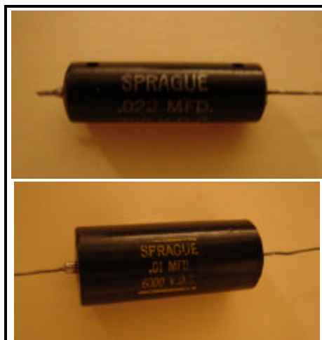
Two early Black Beauties. Note the solder blob and fill tube at the left lead of each capacitor-prime paths for dielectric leakage.
